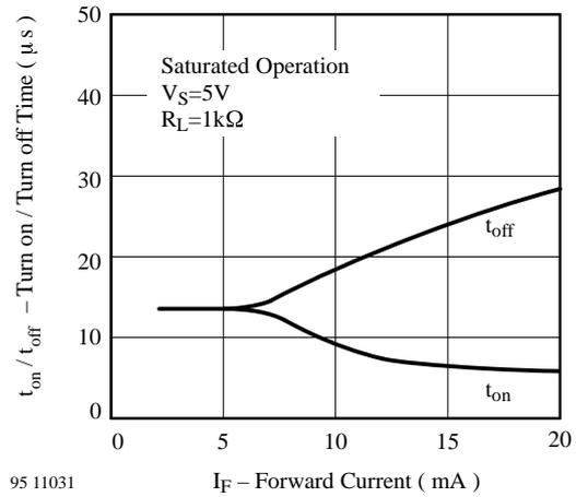
Figure 11. Turn on / off Time vs. Forward Current
