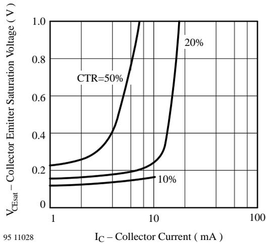
Figure 9. Collector Emitter Sat. Voltage vs. Collector Current
