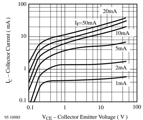
Figure 8. Collector Current vs. Collector Emitter Voltage
