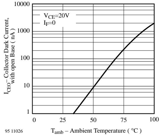
Figure 6. Collector Dark Current vs. Ambient Temperature
